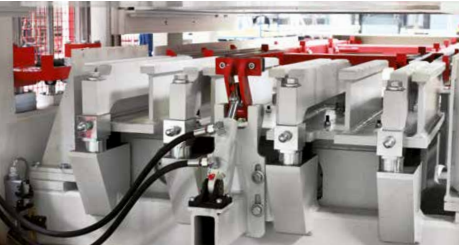
Vibrating table RH 500-3 with impact strips for optimal compaction performance
